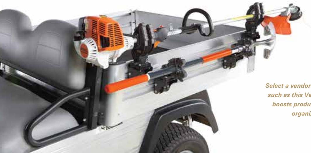
*Select a vendor with a wide range of commercial accessories, such as this VersAttach™ bed-based attachment system that boosts productivity and versatility. The system helps crews organize and protect gear and it reduces round trips.*
