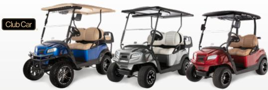
**Electric Onward PTVs** feature smart chargers that issue alerts to prevent common user errors. The vehicles are also available with optional on-board chargers and reel retractors that allow for opportunity charging at any 110-volt outlet. (Images shown include optional upgrades.)
