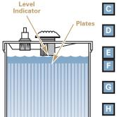
Maintain electrolyte level from at least 1/2-inch (13 mm) above plates to 1/4-inch (6 mm) below level indicator.
