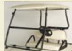
ICS (Integrated Comfort System) Note: Rounded canopy, angled windshield frame and one-piece seat back.
