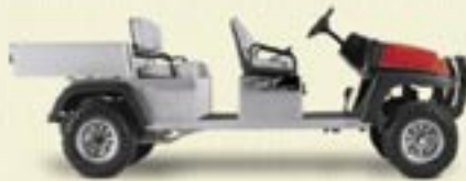
XRT/Pioneer 1200 SE, Carryall 472 Note: 4-passenger configuration and hand brake.
