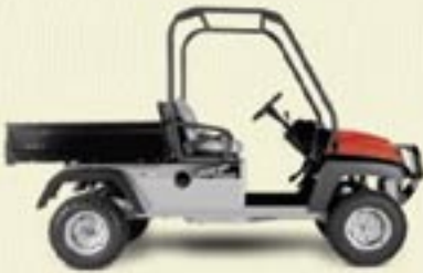
XRT 1500, Carryall 294 Note: ROPS cage and floor-mounted parking brake.
